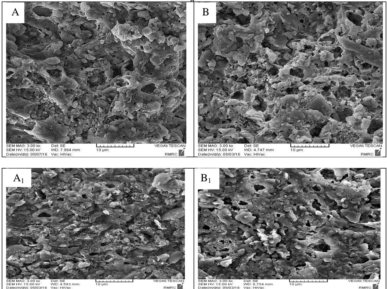
Fig. 4: Scanning electron micrograph of filter samples (A, B) 10% of sawdust and rice husk in slip casting and (A<sub>1</sub>, B<sub>1</sub>) 10% of sawdust and rice husk in pressing.
